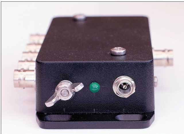
Fig. 2: A side view showing the 2.5 mm coaxial power socket and earth connection.
